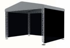
The MILOS MR0 NGW 6x5m aluminium roof incorporates our HD Multi-Cube, eliminating the need for any wires or corner braces for this set-up. Using HD Multicube in the construction of this roof allows loading capacity of up to 30 kg/m plus 200kg for the PA. Great size, simple set-up, no hassle.
