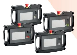
Each EXE Sense / B / D / S series controller has its own wired touch screen remote control
